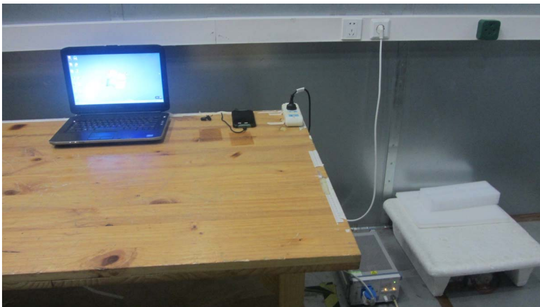
Picture 3 Conducted Emission Test Setup
