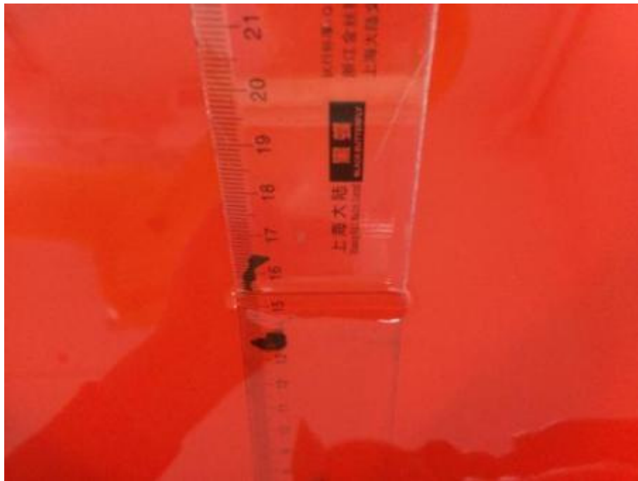
Picture 7-5: Liquid depth in the Flat Phantom (1900 MHz Body)
