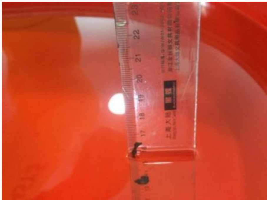
Picture 7-6: Liquid depth in the Flat Phantom (2450 MHz Body)
