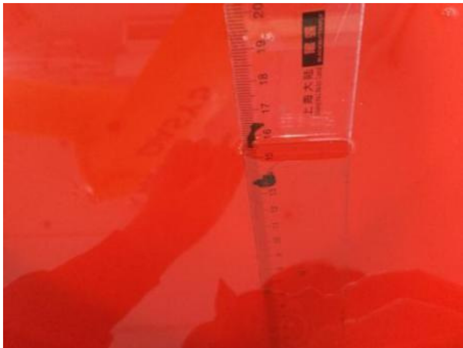
Picture 7-4: Liquid depth in the Flat Phantom (835 MHz Body)
