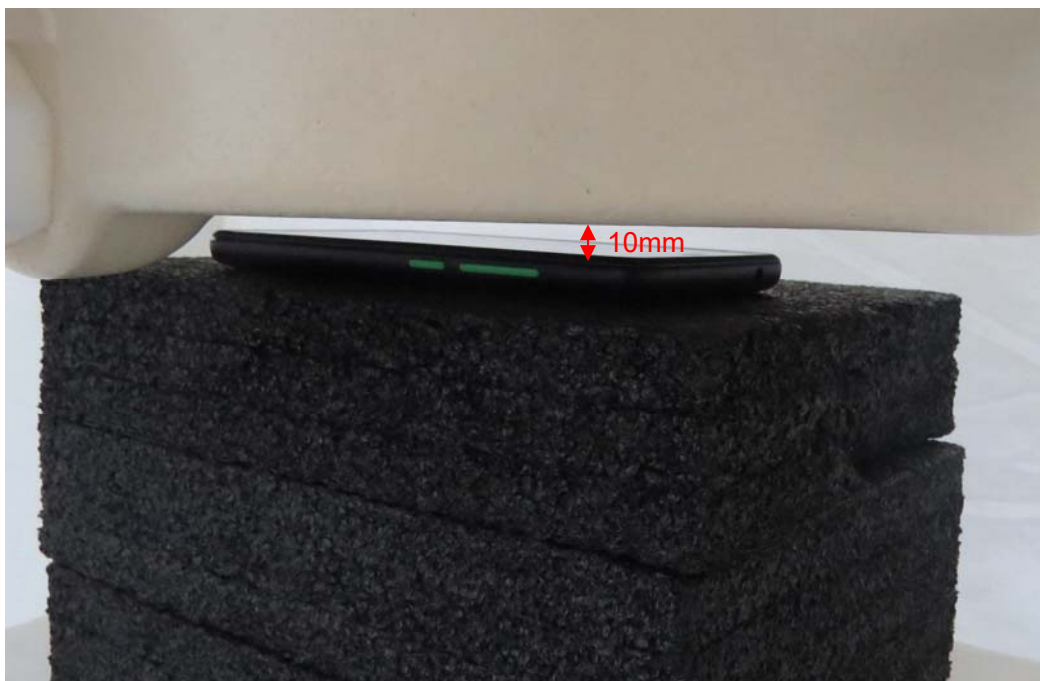
Picture 3: Front Side, the distance from handset to the bottom of the Phantom is 10mm
