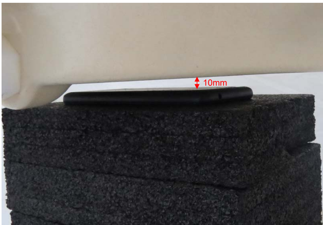
Picture 2: Back Side, the distance from handset to the bottom of the Phantom is 10mm
