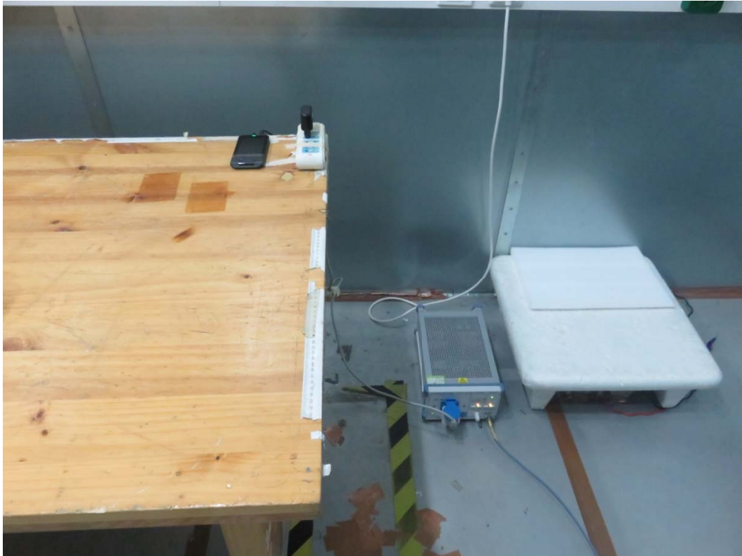
Picture 3 Conducted Emission Test Setup
