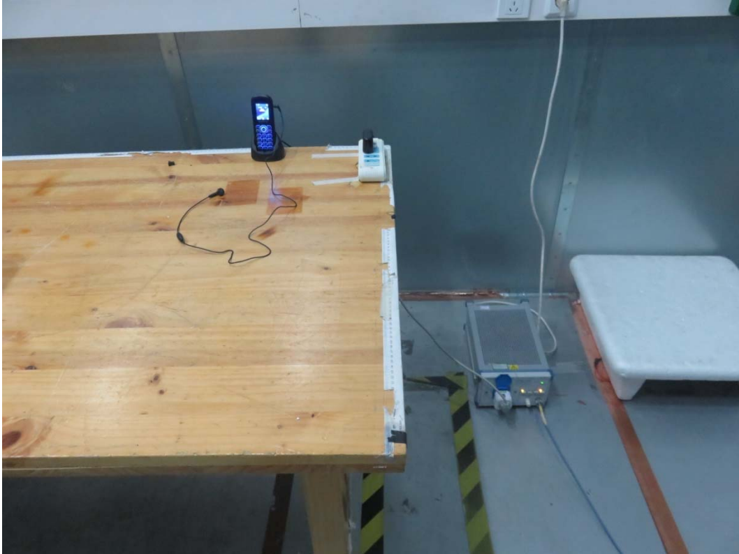
Picture 3 Conducted Emission Test Setup
