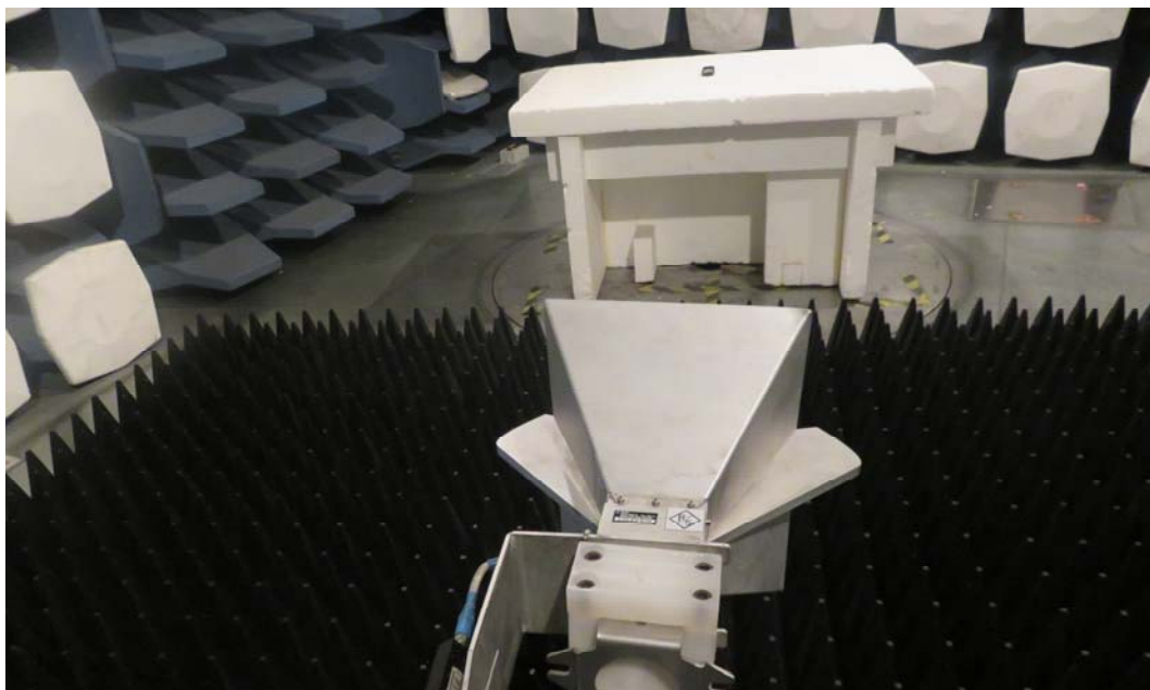
Picture 2: Radiated Spurious Emissions Test setup
