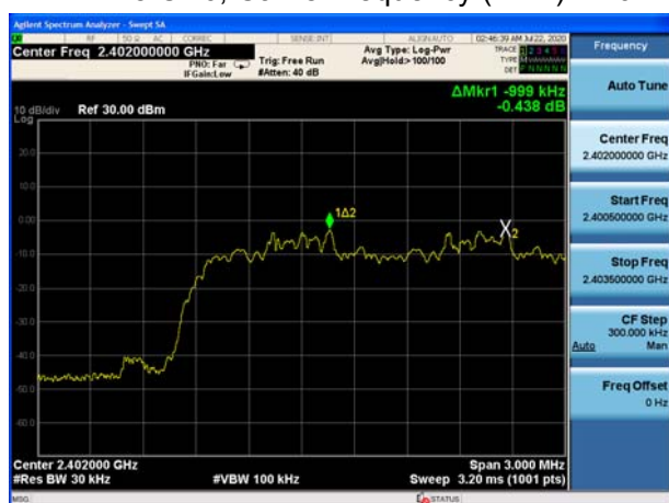
BT 2DH5 CH39, Carrier frequency (MHz): 2441
