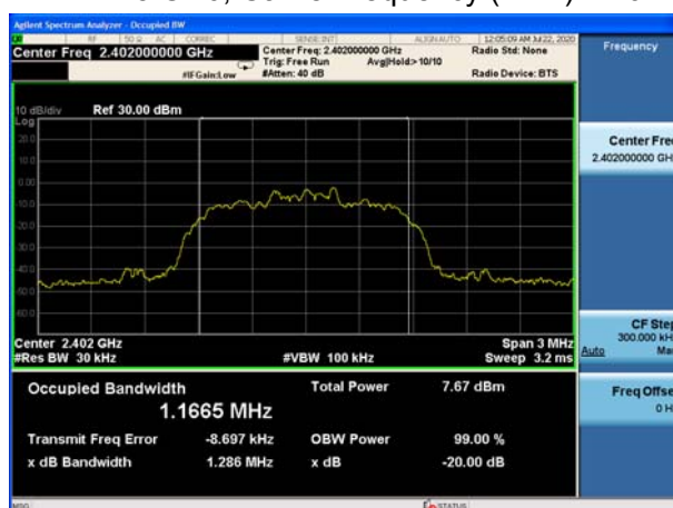
BT 2DH5 CH39, Carrier frequency (MHz): 2441
