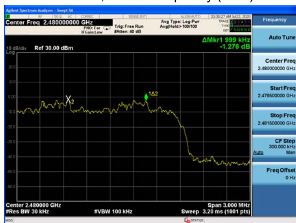
BT 2DH5 CH78, Carrier frequency (MHz): 2480
