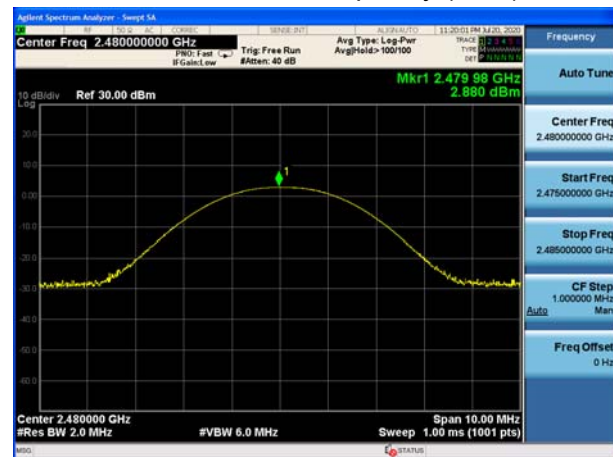
BT DH5 CH78, Carrier frequency (MHz): 2480
