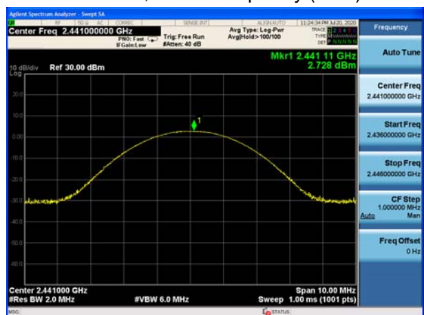
BT 2DH5 CH78, Carrier frequency (MHz): 2480
