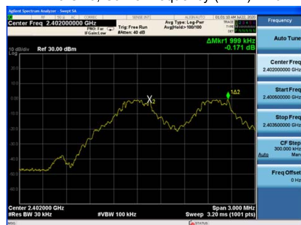
BT DH5 CH39, Carrier frequency (MHz): 2441
