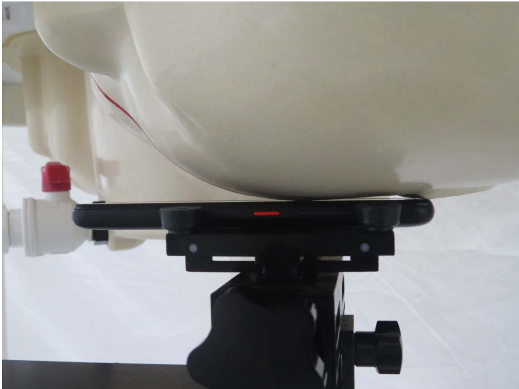
Picture 1: Left Hand Touch Cheek Position
