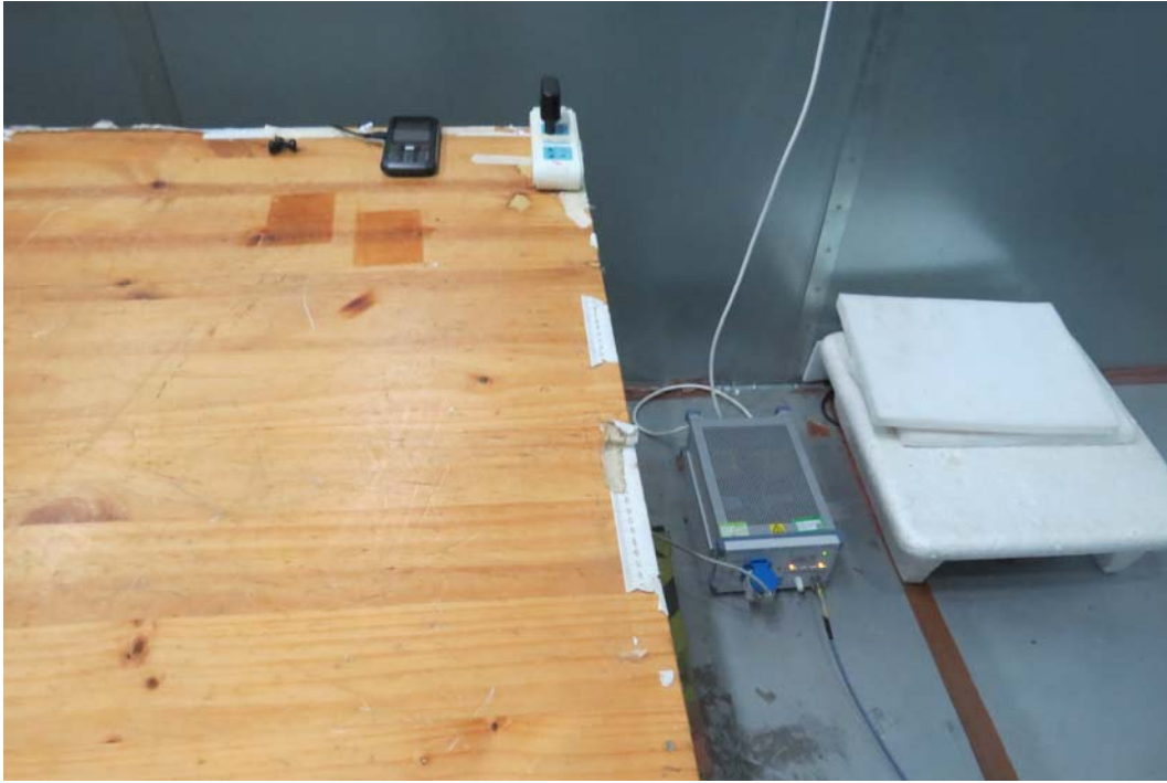
Picture 3 Conducted Emission Test Setup
