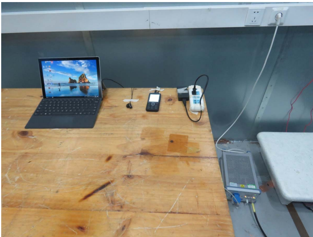
Picture 2 Conducted Emission Test Setup
