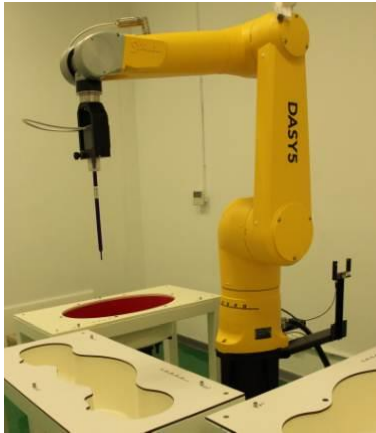
Picture D.6 DSY5 system Set-up
