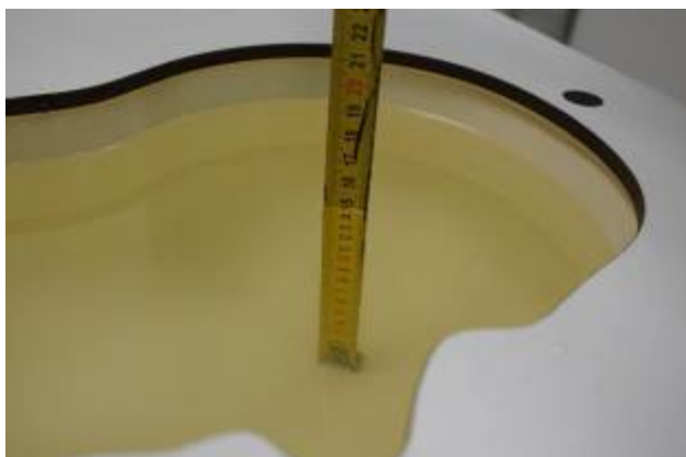
Liquid depth in the head Phantom (5GHz 15cm depth)
