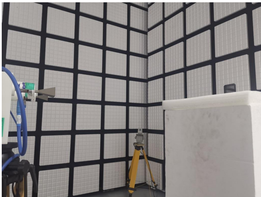
Description: Radiated Emission Test Setup (Above 18GHz)
