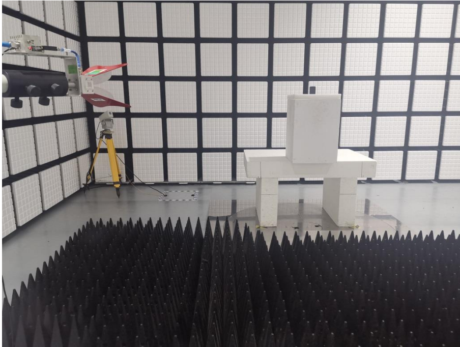
Description: Radiated Emission Test Setup (1 GHz -18GHz)
