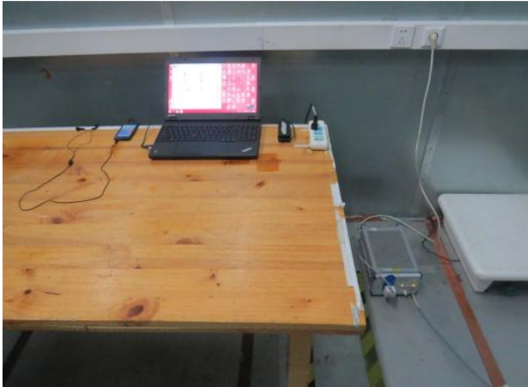
Picture 3 Conducted Emission Test Setup
