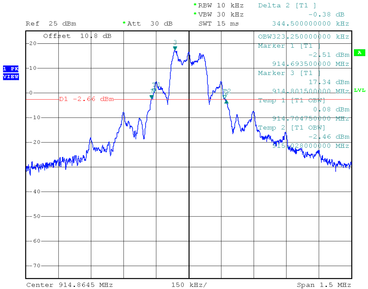
Plot 1. 2 – 20dB Bandwidth and 99% Bandwidth Middle Channel
