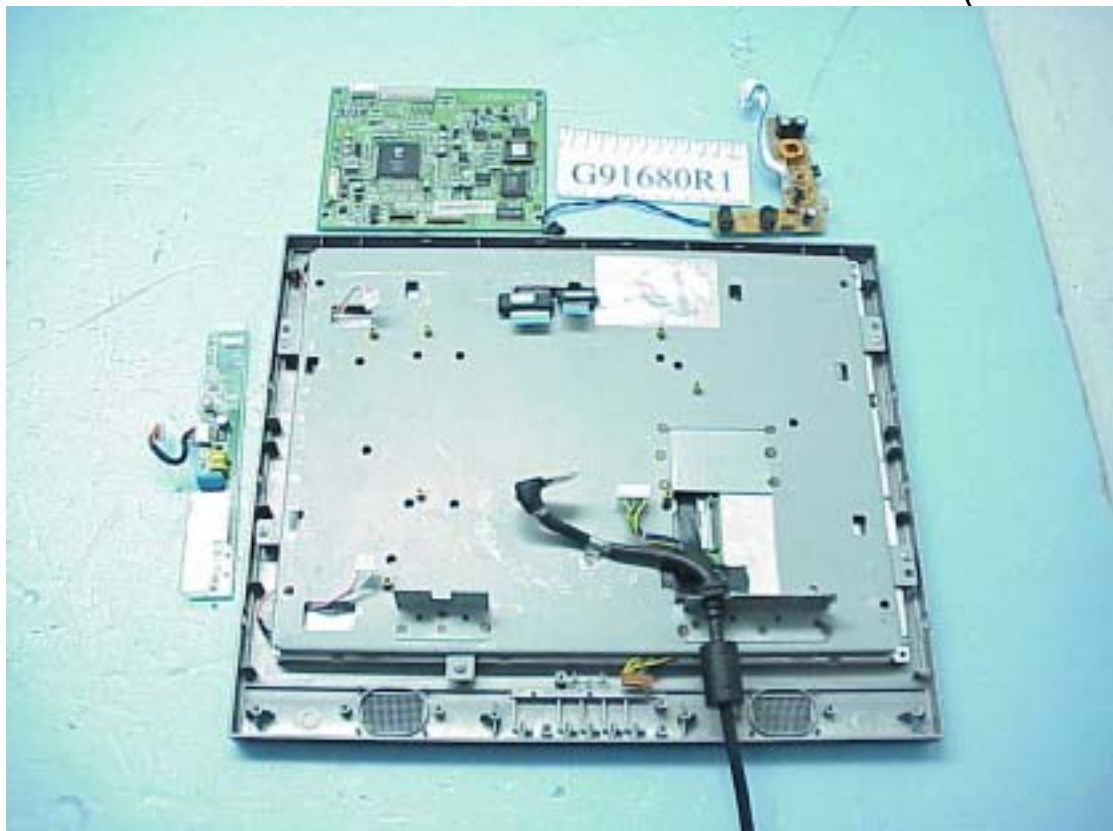
Figure 12 Frame of Internal (Removed PCB)
