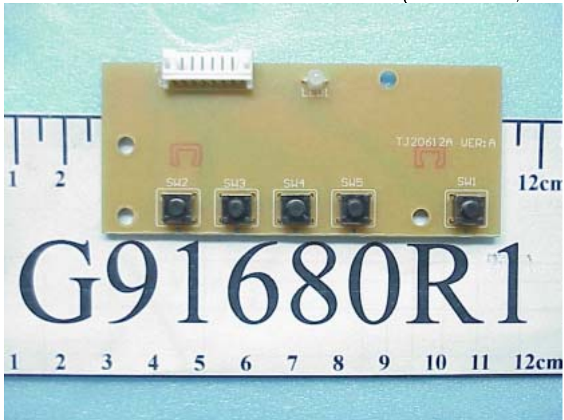
Figure 9 Frame of Internal (Control Board, Front Side)
