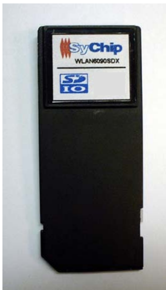
Figure 1 Sychip Combo function SDIO NIC (reference picture only)
