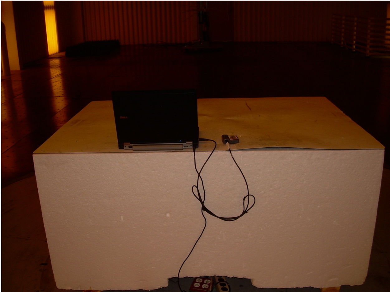
Photograph 2 – Back View Radiated Disturbance Worst Case Configuration – Horizontal
