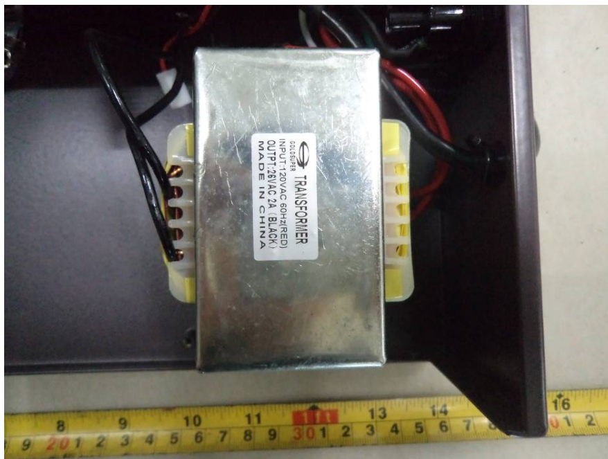
EUT –Transformer View (DC Power)
