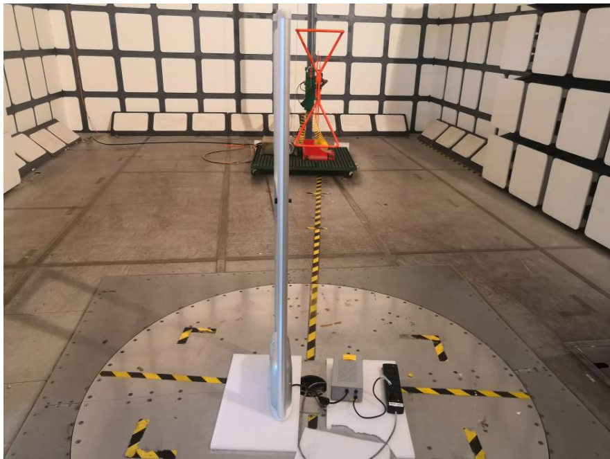
Radiated Emissions - Rear View (30 MHz ~ 1 GHz)
