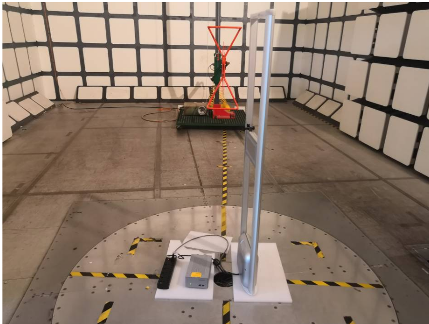
Radiated Emissions - Front View (30 MHz ~ 1 GHz)
