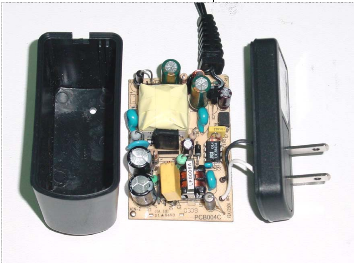
Inside View of Power Adapter
