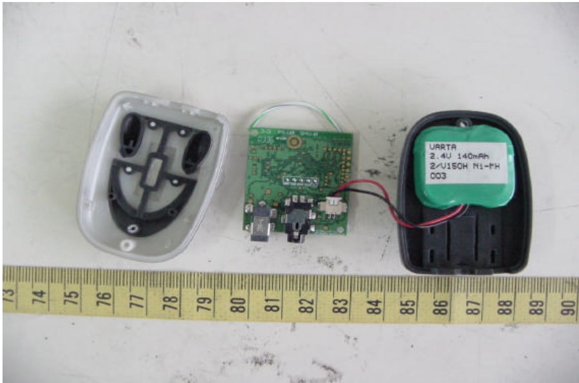
Internal View of EUT
