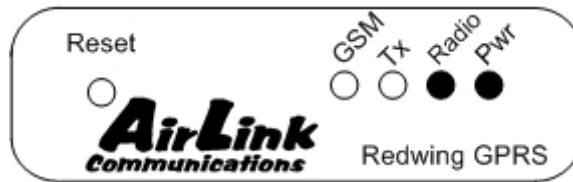
Indicating no GSM/GPRS coverage or no SIM installed
