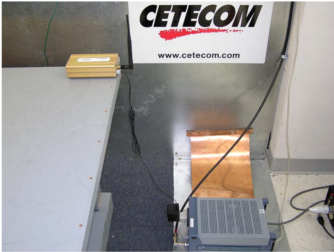
Test setup – AC Line Conducted Emissions Pinpoint
