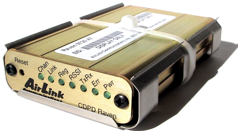
Figure 1 - Raven Mounted in Mounting Bracket
