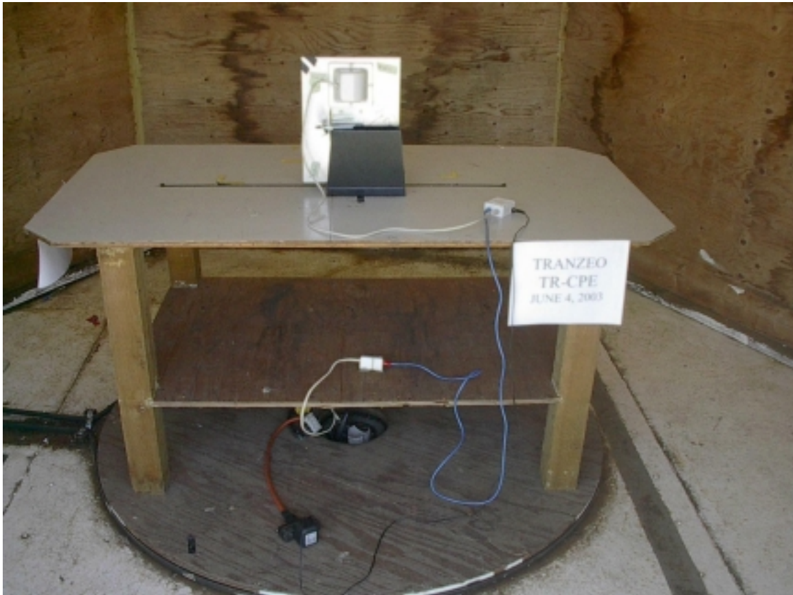
Rear Emissions Test Setup
