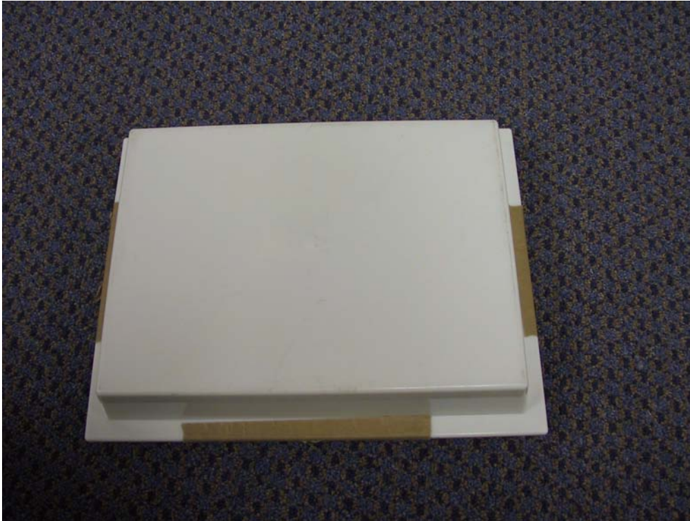
External front of unit, 15 dBi and N Connector
