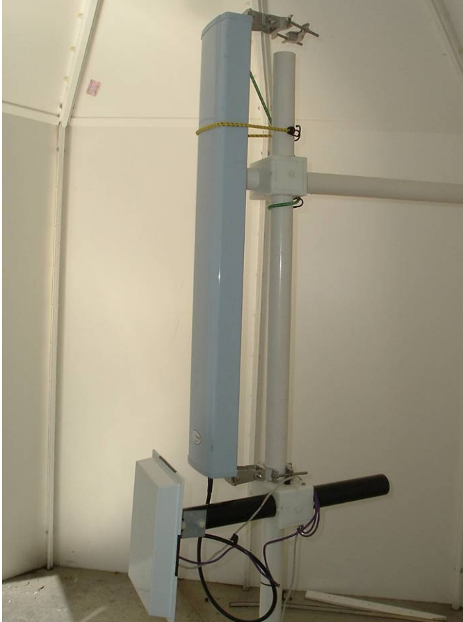
TR-CPE90-Nf with 17 dBi Sector Antenna
