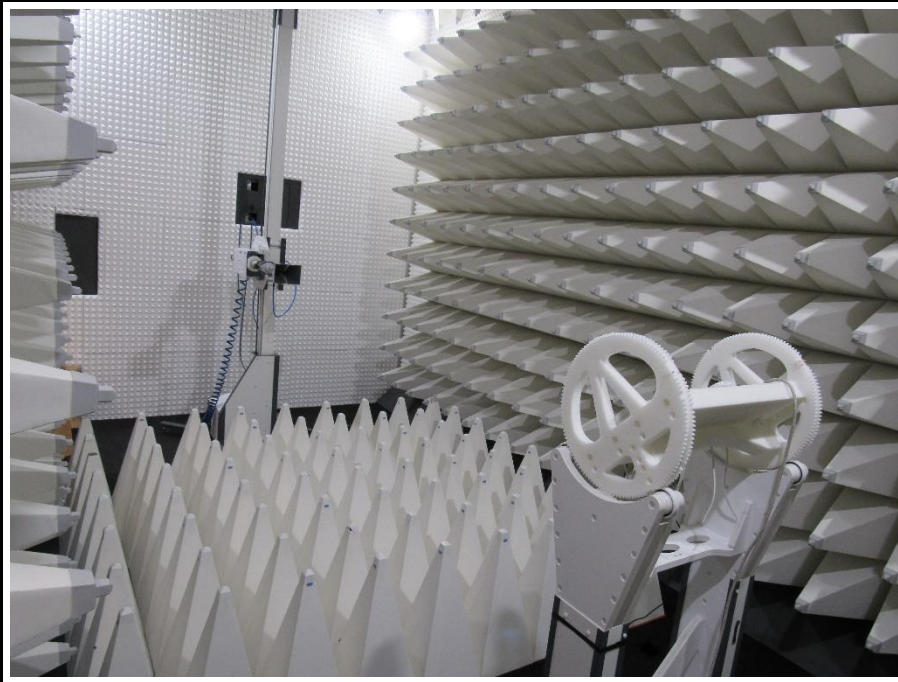
Setup above 1 GHz
