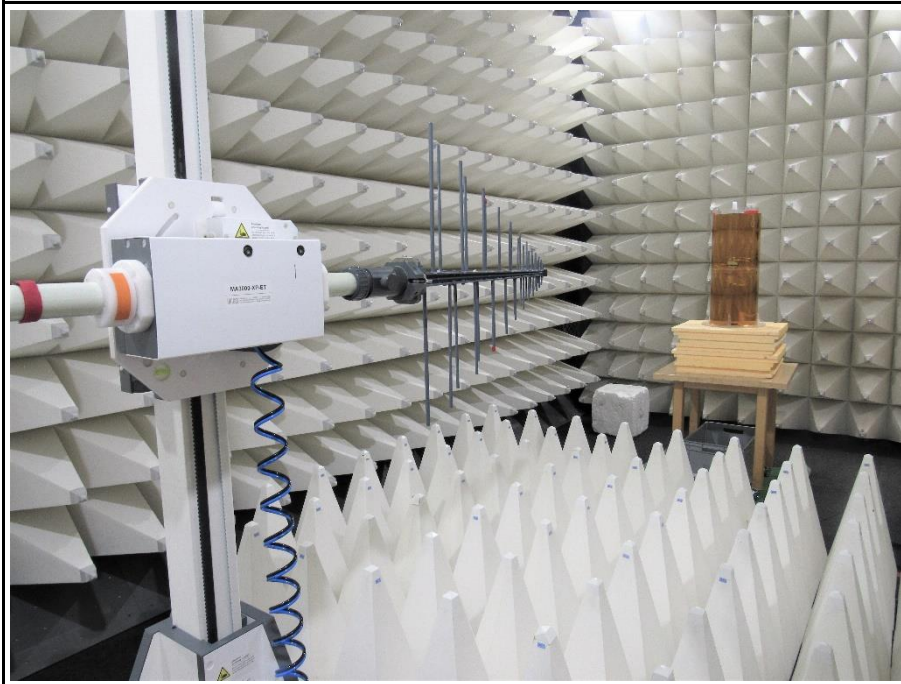
Test setup – Antenna pattern measurement
