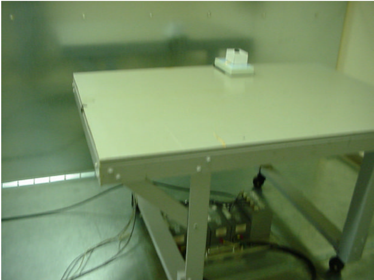
Figure 17 - Conducted Emissions Test Setup (Front) CUI Stack Model DSA-0151A-12
