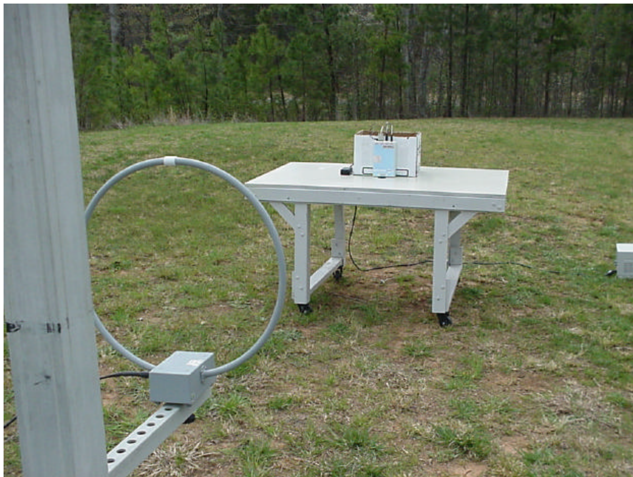
Figure 14 - Radiated Emissions Test Setup (9KHz to 30 MHz)
