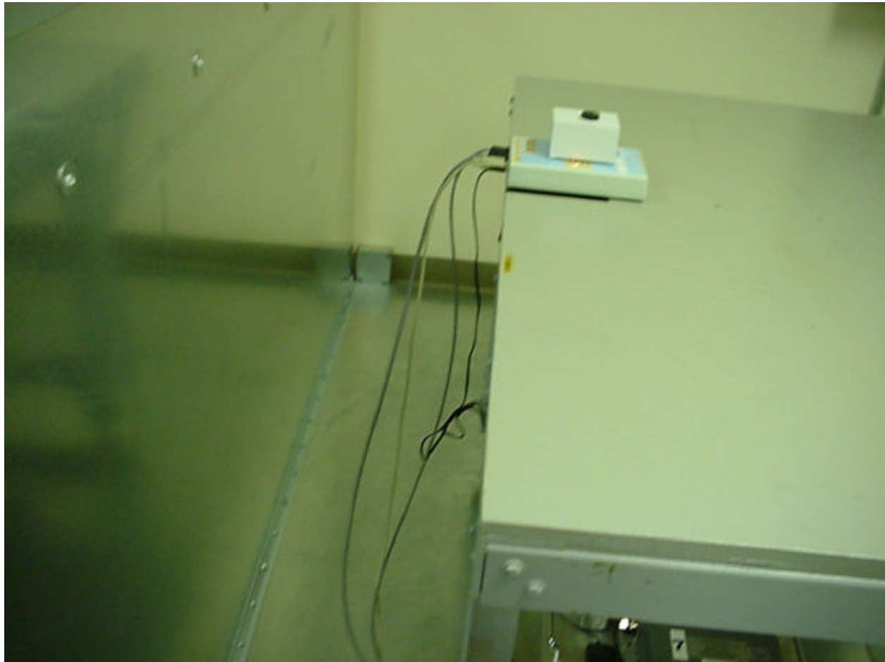
Figure 18 - Conducted Emissions Test Setup (Back) CUI Stack Model DSA-0151A-12
