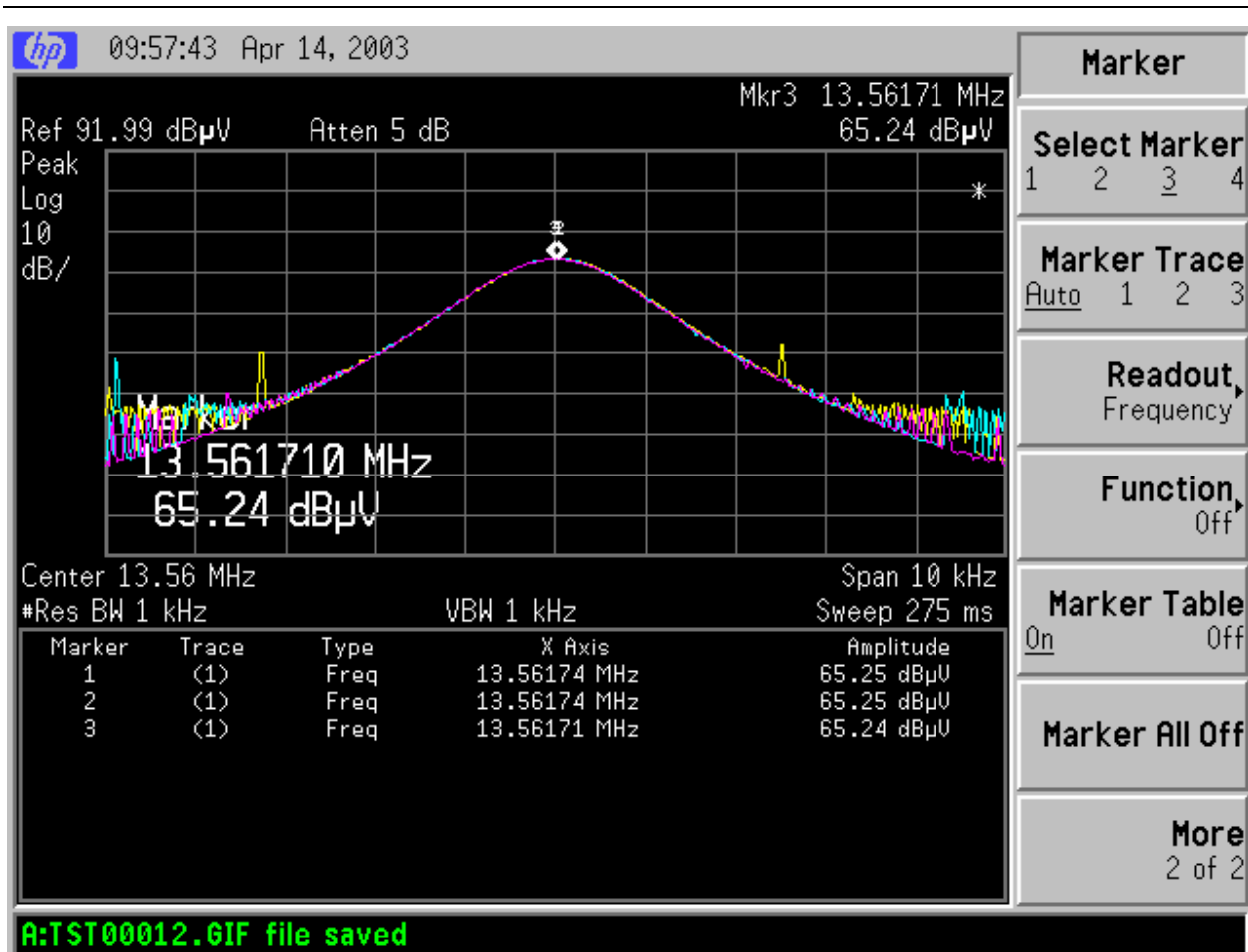
Figure 20 – Primary Supply Voltage Variation from 85% to 115% of nominal voltage
