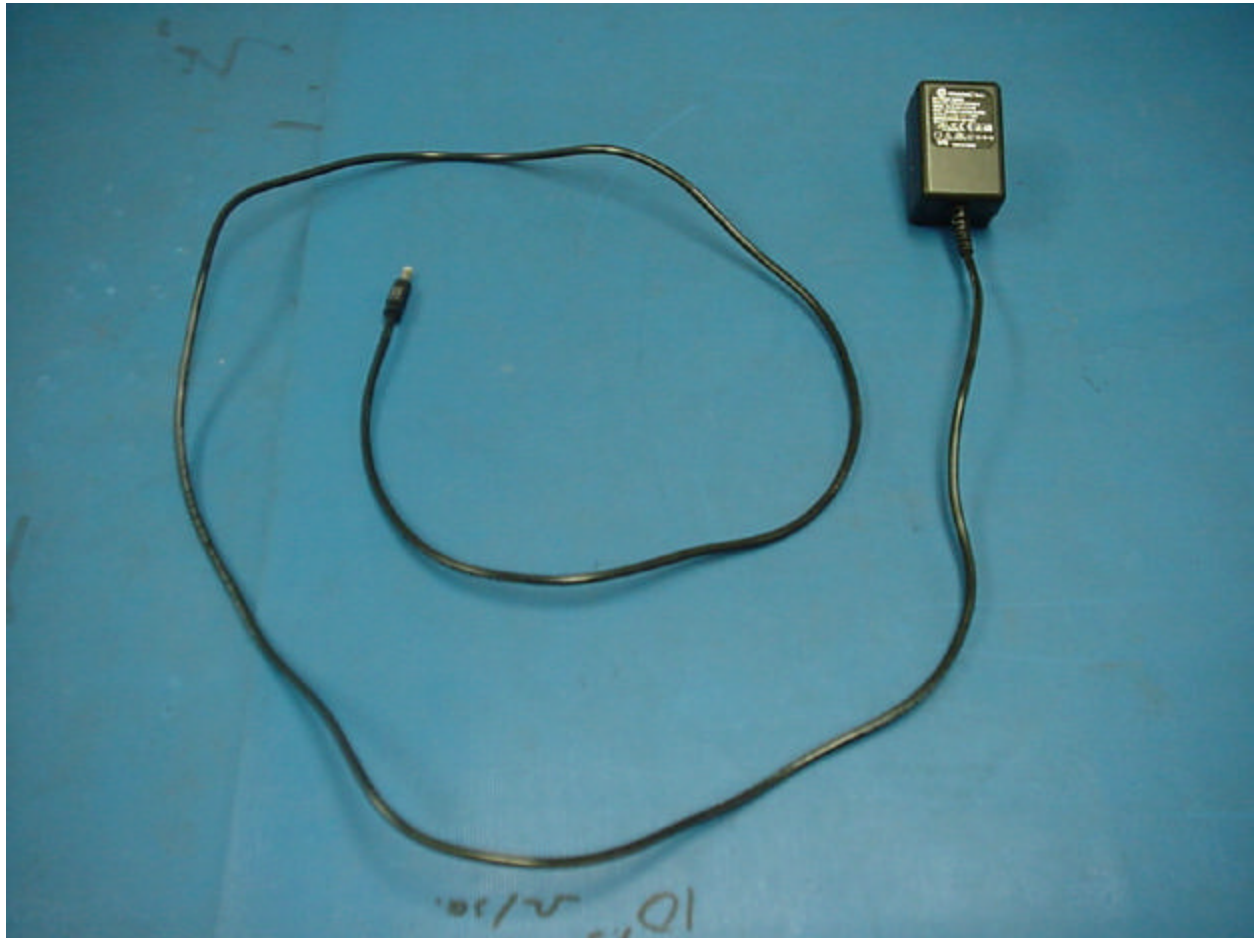
Figure 15 – Photo of the power supply
