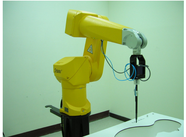
Fig. 5.2 Probe setup on robot
