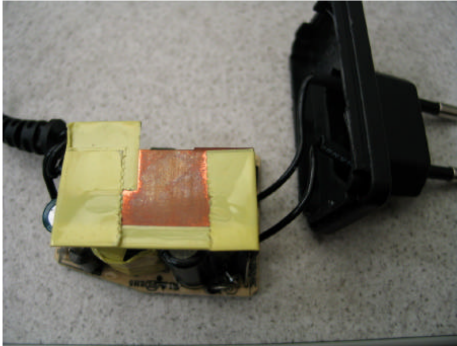
Picture 7 : AC/DC supply for the cradle (top view of the PCB)
