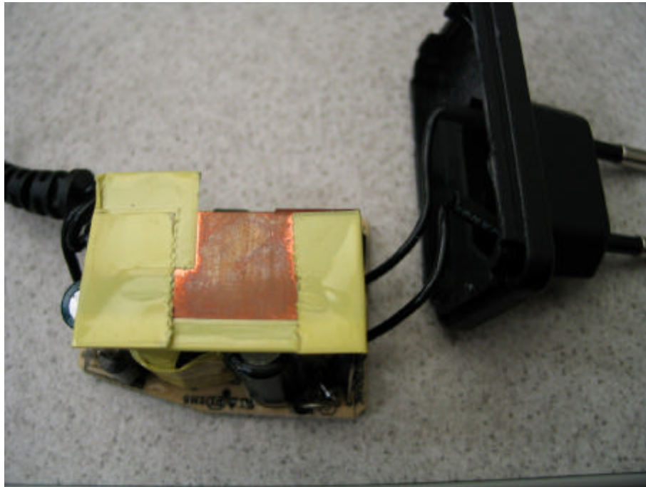
Picture 7 : AC/DC supply for the charging station
