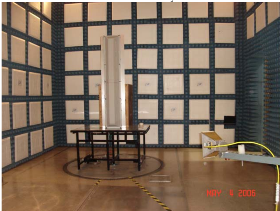
Test Setup For Measurement of Radiated Emissions Horizontal Polarity
