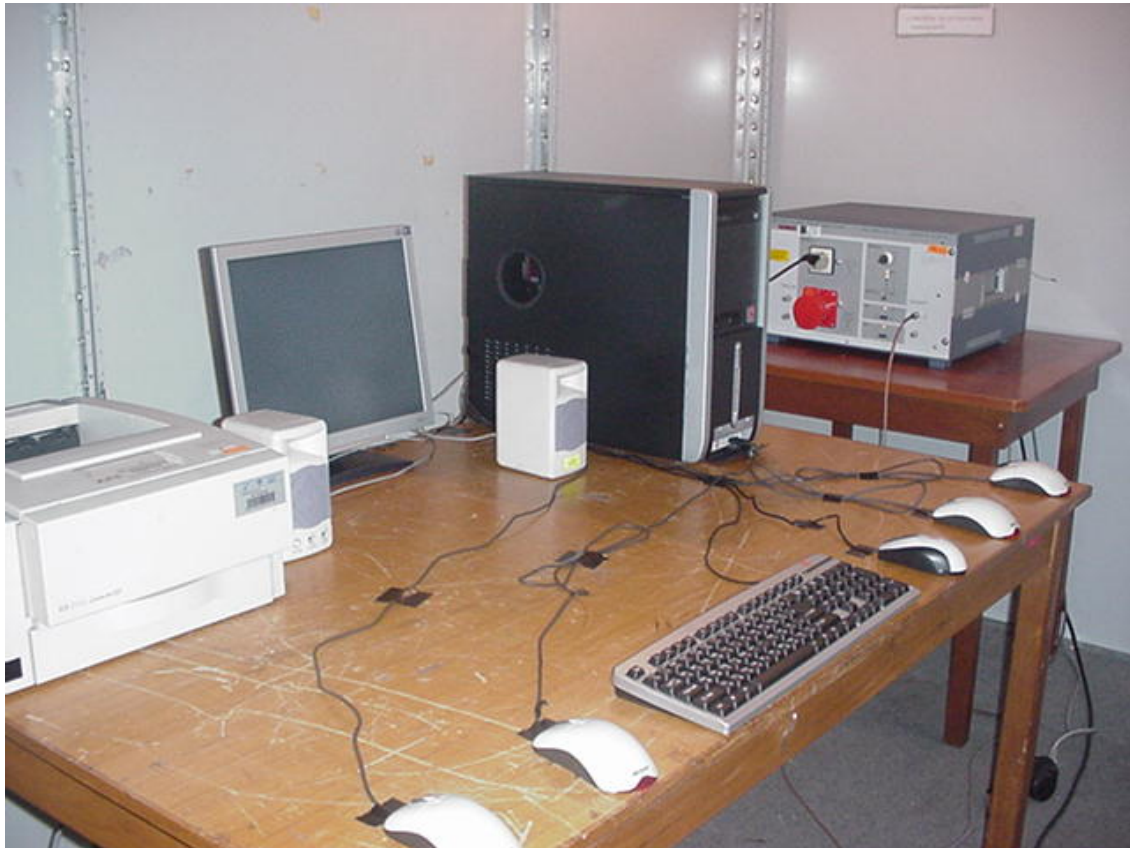
Figure 1-Conducted emission test set up
