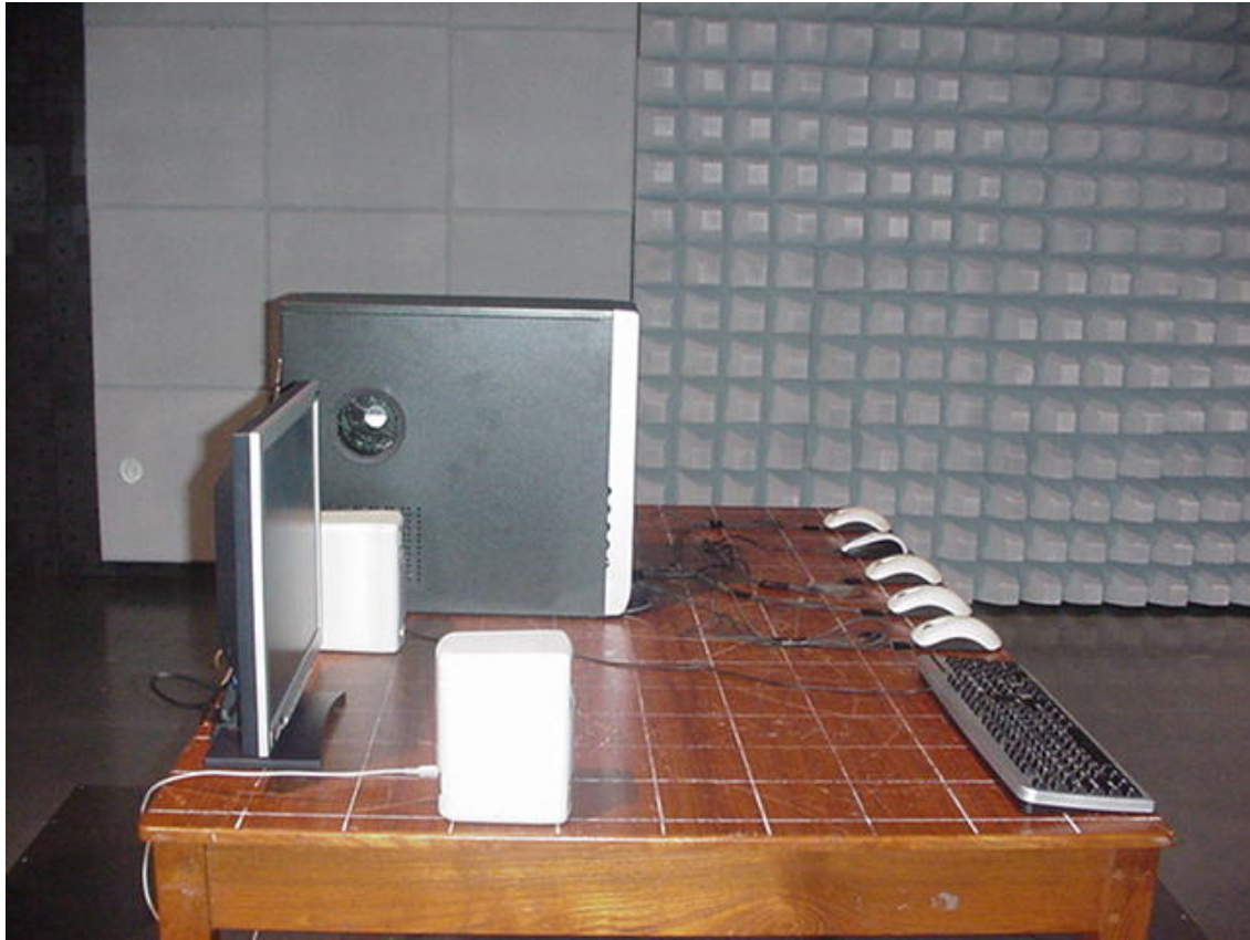
Figure 3-Radiated emission Test set up (side view)
