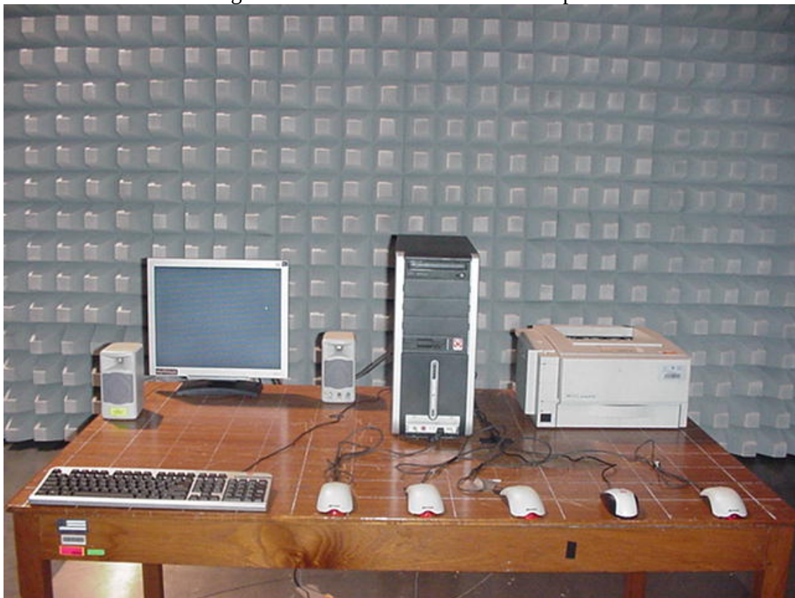
Figure 2-Radiated emission test set up
