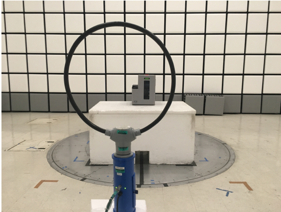
Radiated Spurious Emissions Below 30 MHz Front
