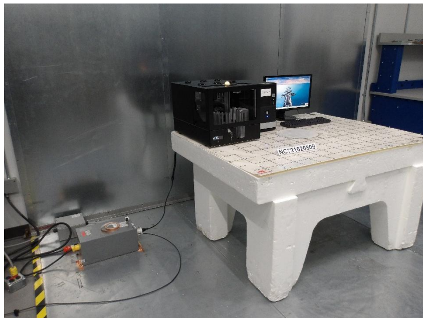
Figure 5.1 – Power Line Conducted Emission – Front View
