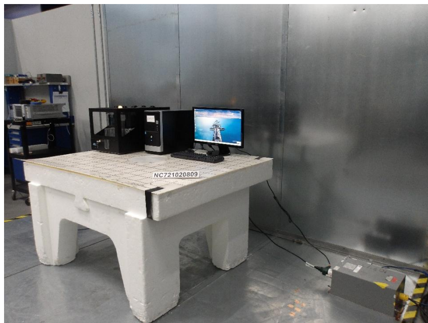
Figure 5.2 – Power Line Conducted Emission – Front View
