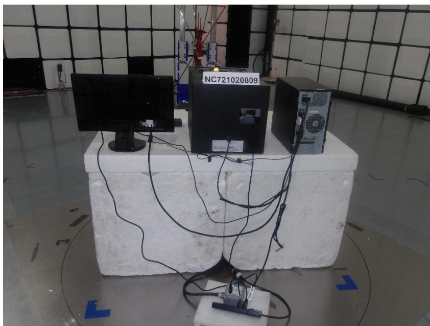
Figure 4.4 – Radiated Spurious Emission 30MHz – 1GHz– Rear View
