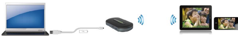
PNY works as a WiFi SD reader or USB external HDD
