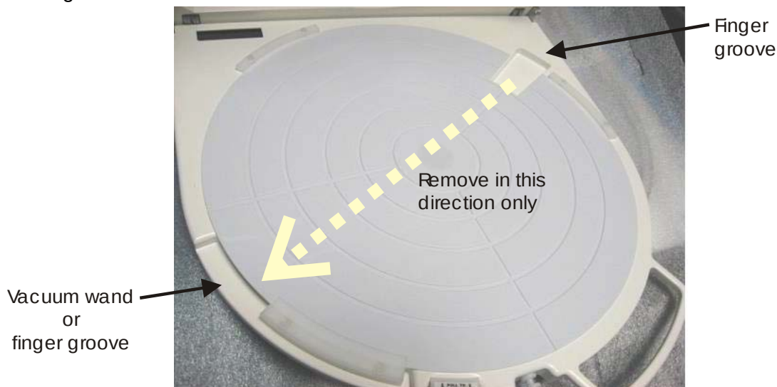
Figure 3-9 Wafer Removal Points
