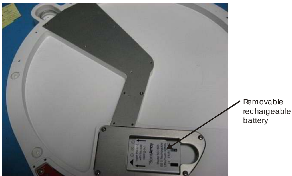
Figure 3-3 Backside of C/C Carrier
