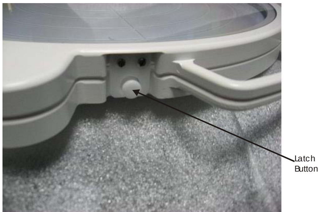
Figure 3-6. Unlatching the Carrier Station
