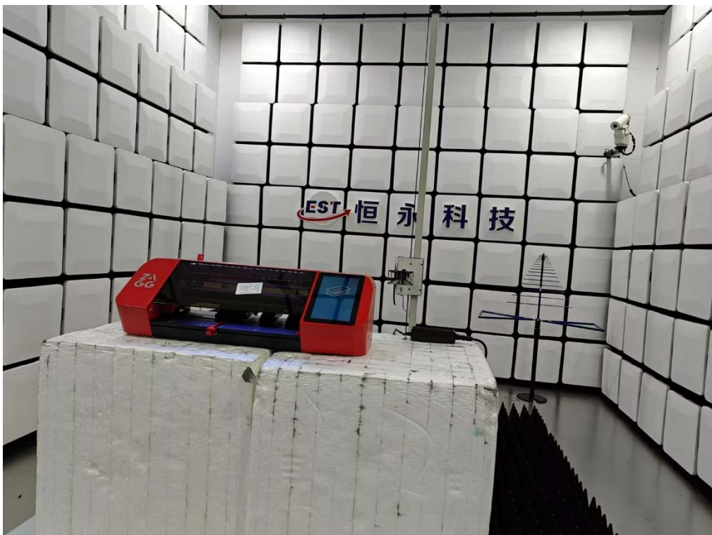
Radiated Test (Above 1GHz)
