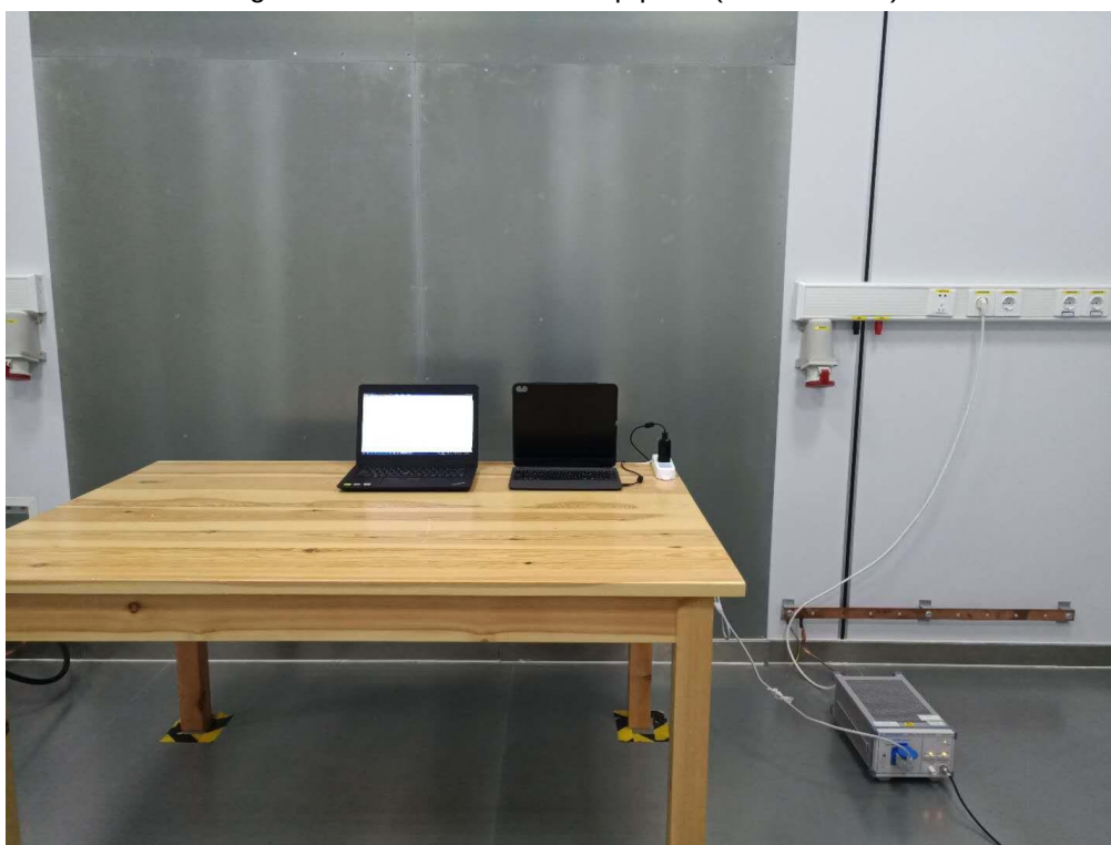
Fig. 4 Power line conducted emission setup photo
