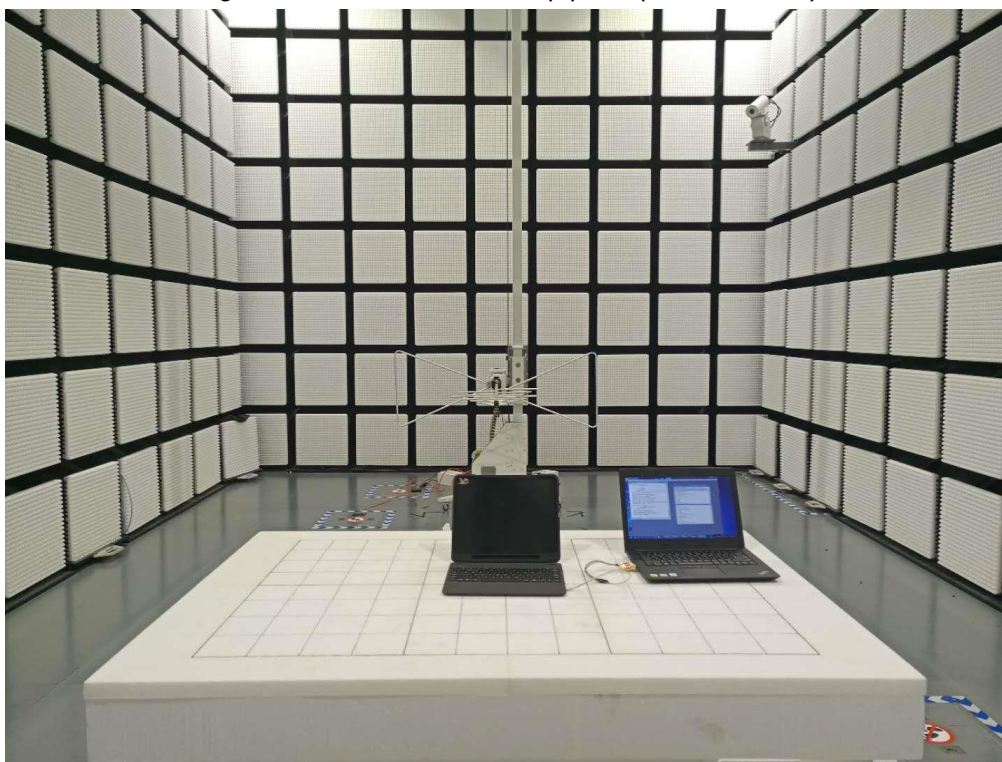
Fig. 2 Radiated emission setup photo(30MHz-1GHz)
