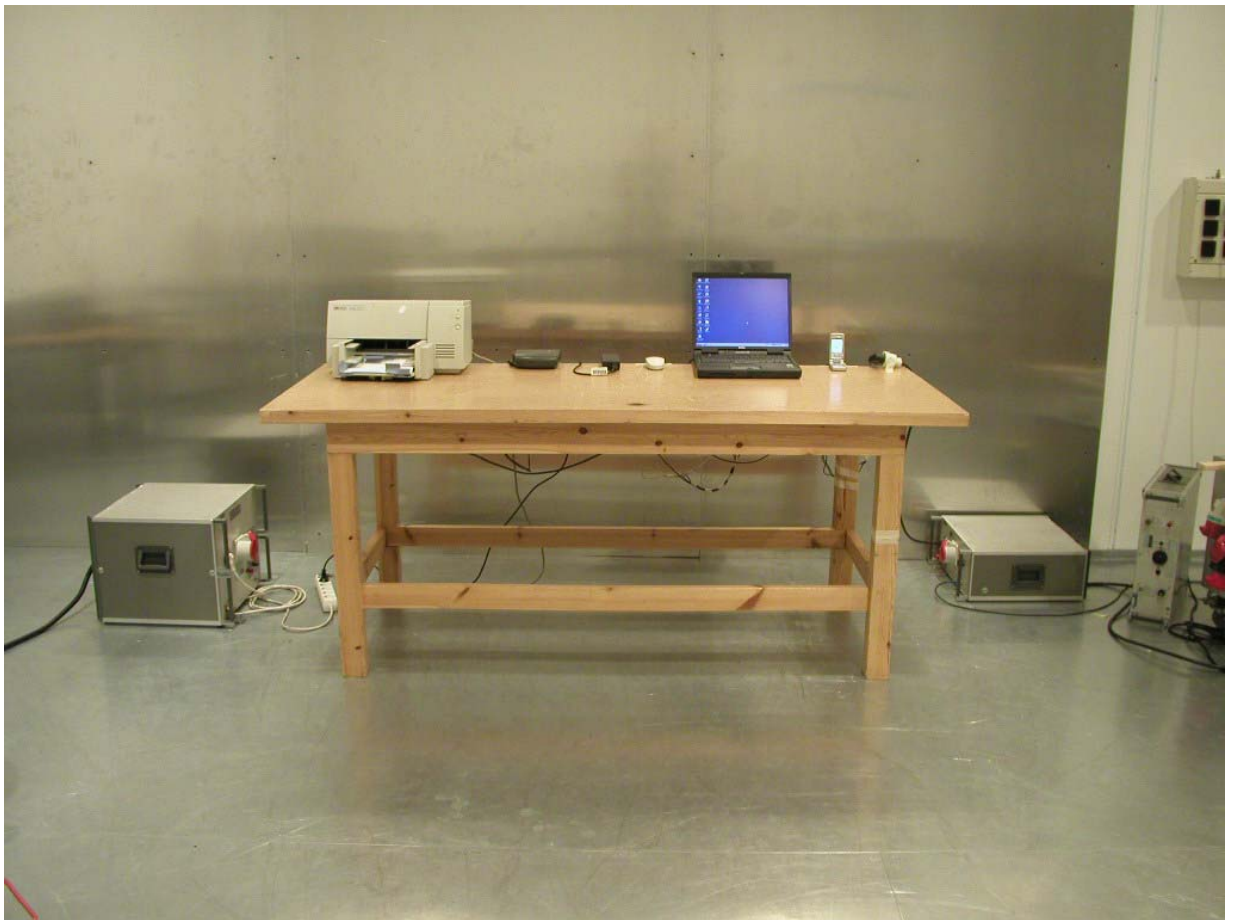
Photograph 1. AC power line conducted emissions test setup
