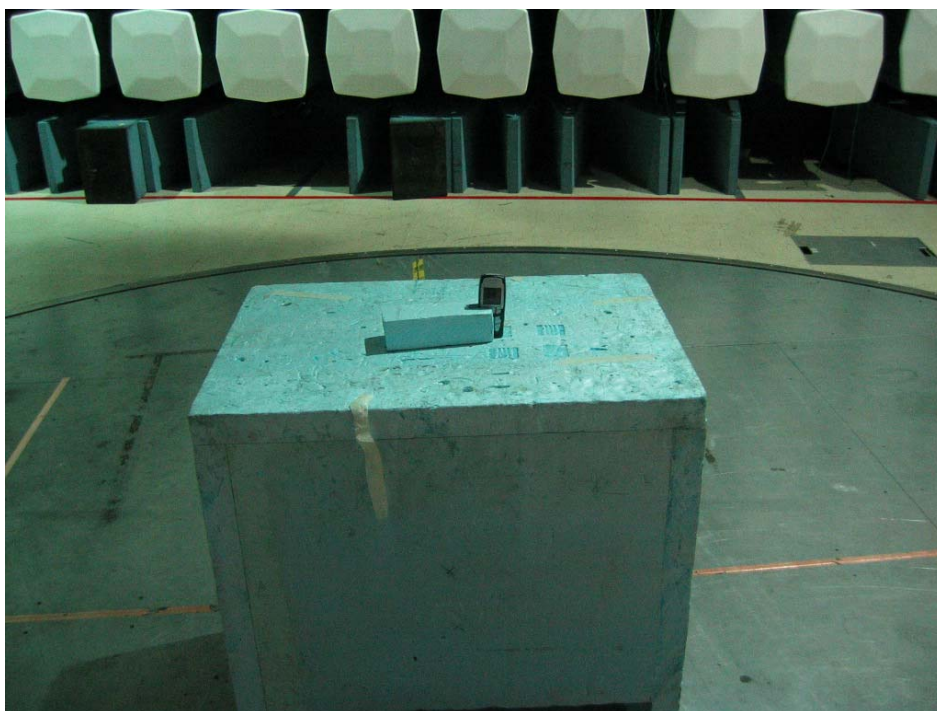
Photograph 1. Spurious radiated emissions test setup
