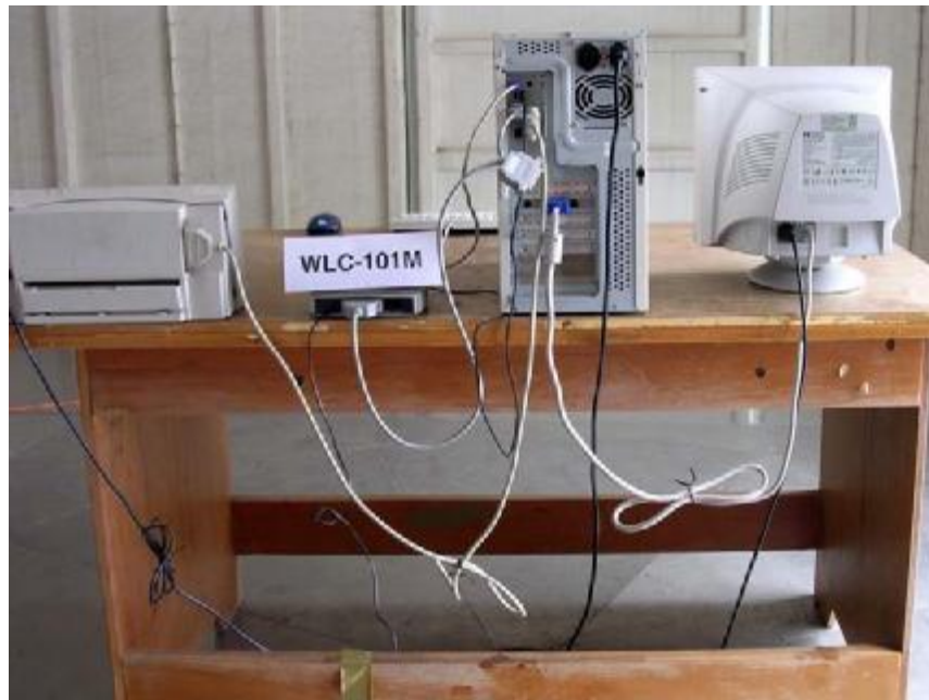
Photo 4: Radiated Emission Test Set-up (rear)
