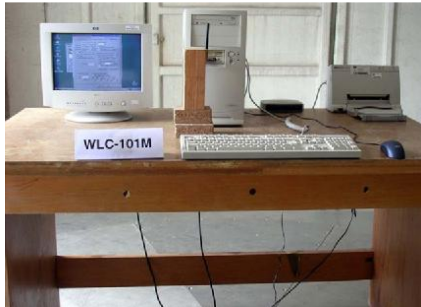
Photo 1: Radiated Emission Test Set-up (front) (ETU with antenna 1)
