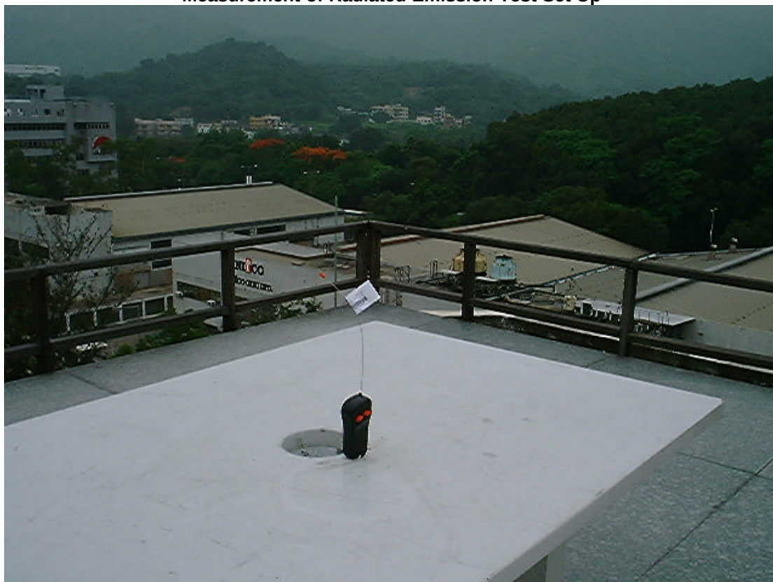
Measurement of Radiated Emission Test Set Up
