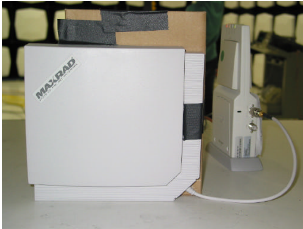
13dBi 2.4 – 2.5 GHz Maxrad MFP24103XFPTMSMA
