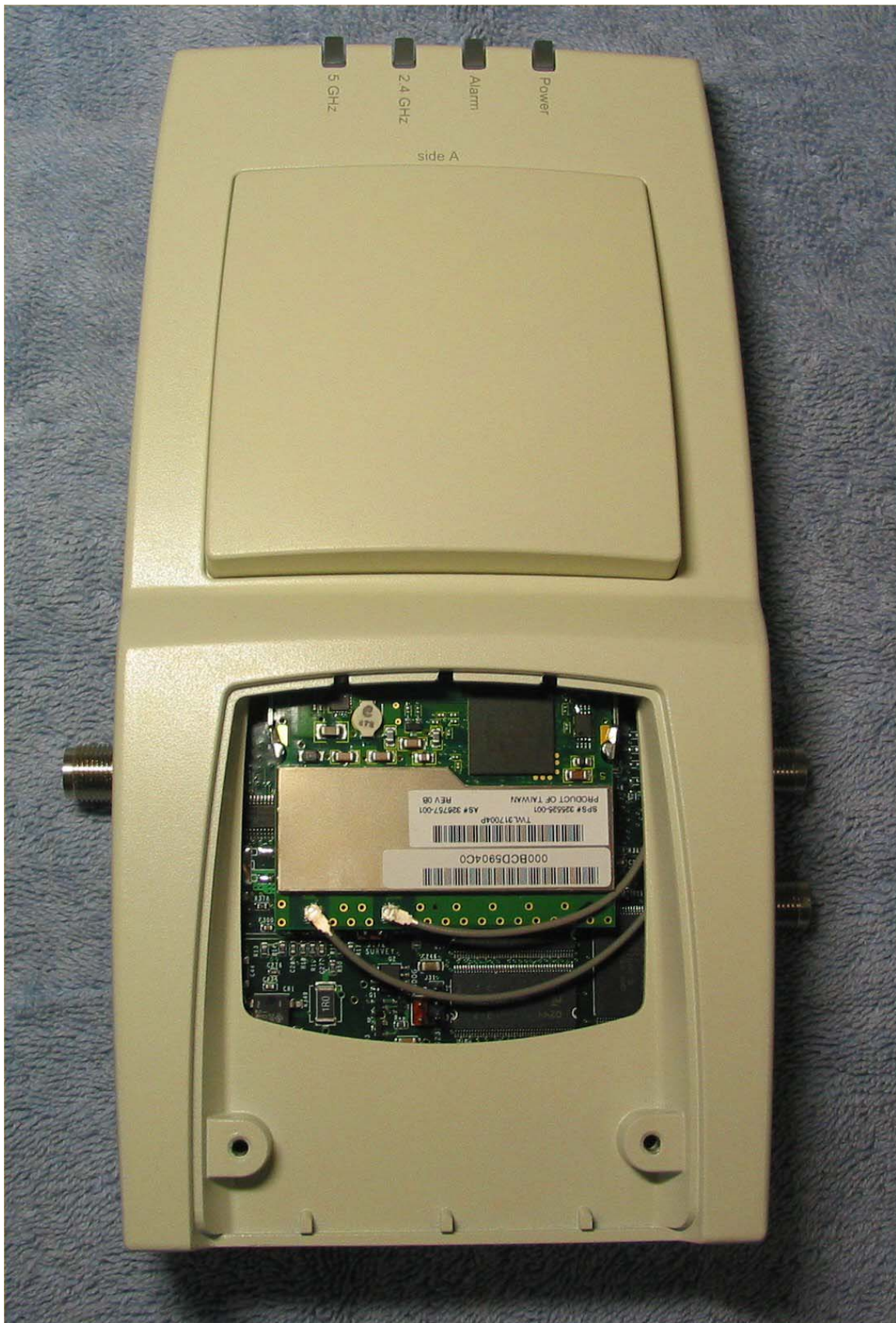
Access point with cover removed
